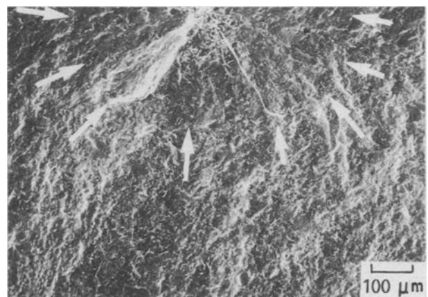
Figure 4. A typical fracture surface showing a well-developed half-penny crack configuration.
